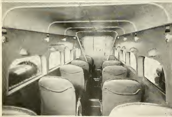
Passengers' cabin of the latest Stinson Model U Trimotor showing the improved seating arrangement for ten passengers
